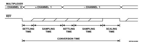
Figure 23. Multiplexer and Conversion Timing—Continuous Conversion on Several Channels with Chopping Enabled
