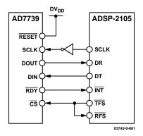
Figure 13. AD7739 to Host Device Interface, DSP
