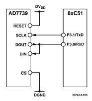
Figure 14. AD7739 to Host Device Interface, 2-Wire Configuration
