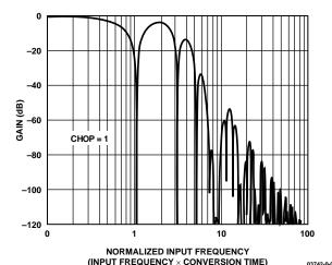
(INPUT FREQUENCY × CONVERSION TIME) 03742-0-026 Figure 25. Typical ADC Frequency Response, Chopping Enabled
