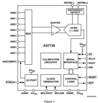
The part is specified for operation over the extended industrial temperature range of  $-40^{\circ}$ C to  $+105^{\circ}$ C.
