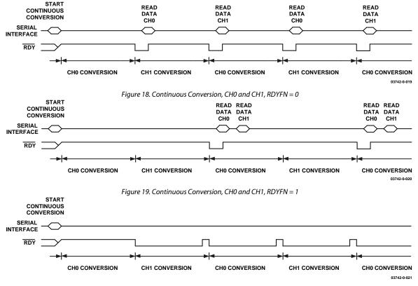
Figure 20. Continuous Conversion, CH0 and CH1, No Data Read
