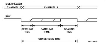
Figure 24. Multiplexer and Conversion Timing—Continuous Conversion on Several Channels with Chopping Disabled
