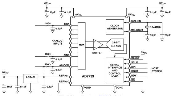
Figure 27. Typical Connections for the AD7739 Application
