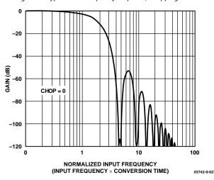
Figure 26. Typical ADC Frequency Response, Chopping Disabled
