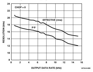
Figure 10. Typical Effective and Peak-to-Peak Resolution; AIN Voltage = 0 V, AIN Range  $\pm$ 1.25 V, Chopping Disabled, MCLK = 6.144 MHz
