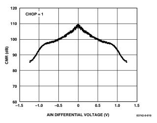
Figure 11. Typical Common-Mode Rejection vs. AIN Voltage; AIN Range  $\pm$ 1.25 V, Conversion Time 397  $\mu$ s, Chopping Enabled, MCLK = 6.144 MHz
