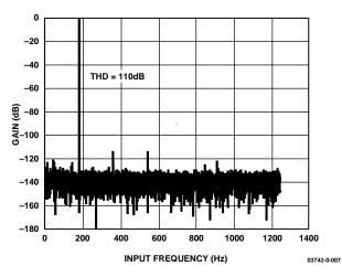
Figure 8. Typical FFT Plot; Input Sine Wave 183 Hz, 1.2 V Peak, AIN Range  $\pm$ 1.25 V, Conversion Time 397 µs, Chopping Enabled, MCLK = 6.144 MHz
