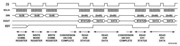
Figure 21. Continuous Conversion, CH0 and CH1, Continuous Read
