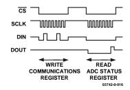
Figure 15. Serial Interface Signals—Registers Access
