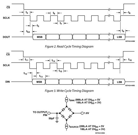
Figure 4. Load Circuit for Access Time and Bus Relinquish Time
