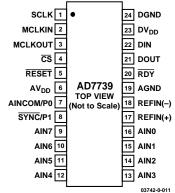
Figure 5. Pin Configuration (24-Lead TSSOP)
