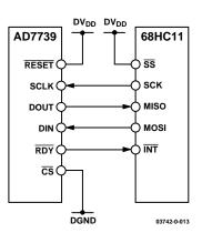
Figure 12. AD7739 to Host Device Interface, SPI
