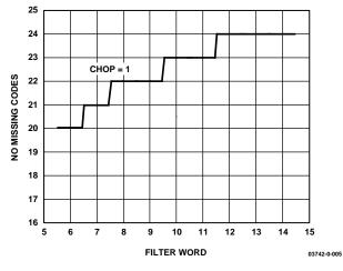
Figure 6. No Missing Codes Performance, Chopping Enabled
