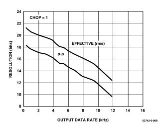
Figure 9. Typical Effective and Peak-to-Peak Resolution; AIN Voltage = 0 V, AIN Range  $\pm 1.25$  V, Chopping Enabled, MCLK = 6.144 MHz
