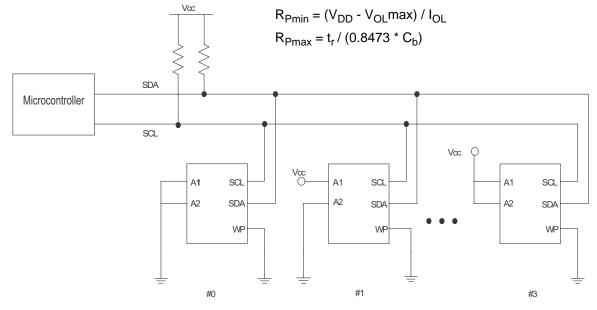
Figure 2. System Configuration using Serial (I<sup>2</sup>C) nvSRAM
