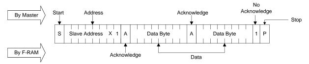
Figure 13. Hs-mode Current Address Read
