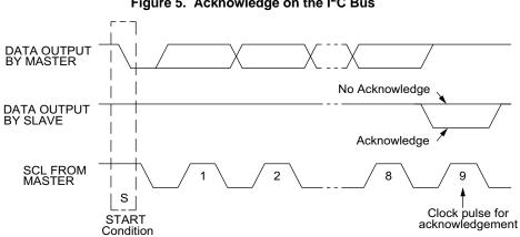
Figure 5. Acknowledge on the I<sup>2</sup>C Bus
