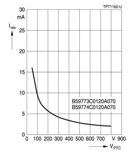
Minimum resistance of PTC thermistors versus applied voltage (pulsed)
