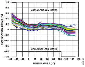
Figure 6. Temperature Accuracy at 5 V
