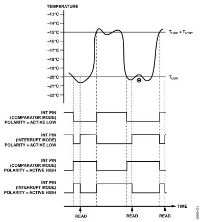
$\textit{Figure 20. INT Output Temperature Response Diagram for T}_{LOW} \, \textit{Undertemperature Events}$
