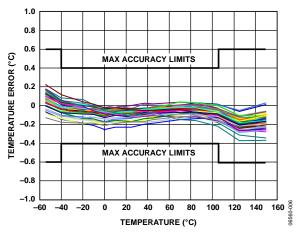
Figure 5. Temperature Accuracy at 3 V
