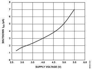
Figure 10. Shutdown Current vs. Supply Voltage at 25°C
