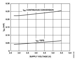
Figure 9. Average Operating Supply Current vs. Supply Voltage at 25  $^{\circ}$ C
