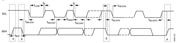
Figure 2. Serial Interface Timing Diagram
