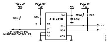
Figure 14. Typical I<sup>2</sup>C Interface Connection
