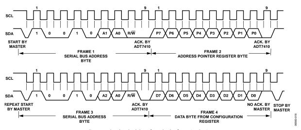
${\it Figure~17. Reading~Back~Data~from~the~Configuration~Register}$
