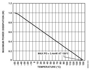
Figure 3. SOIC\_N Maximum Power Dissipation vs. Temperature
