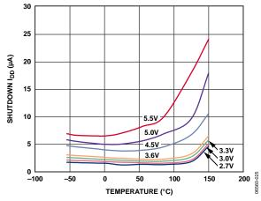
Figure 8. Shutdown Current vs. Temperature
