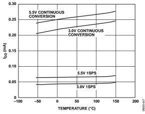
Figure 7. Operating Supply Current vs. Temperature
