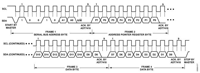
Figure 16. Writing to a Register Followed by Two Bytes of Data
