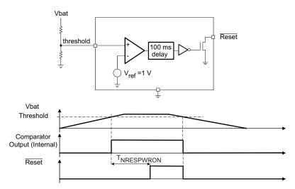
Figure 23. RESET Pulse Circuit for TPS65053x
