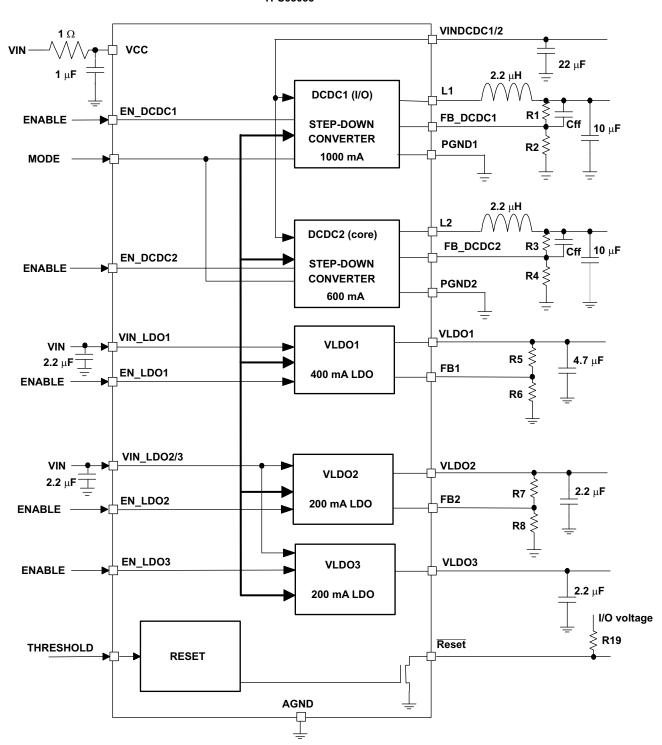
Figure 19. TPS65053 Functional Block Diagram
