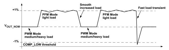
Figure 21. Dynamic Voltage Positioning
