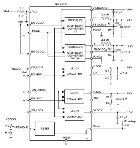
Figure 25. Typical Application Schematic
