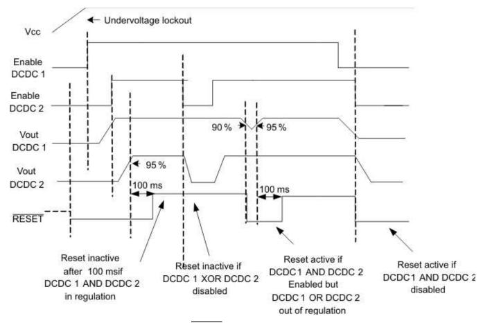
Figure 24. RESET Pulse Circuit for TPS65058
