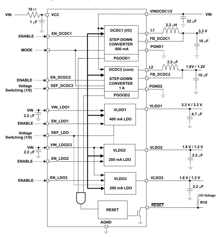
Figure 20. TPS65058 Functional Block Diagram
