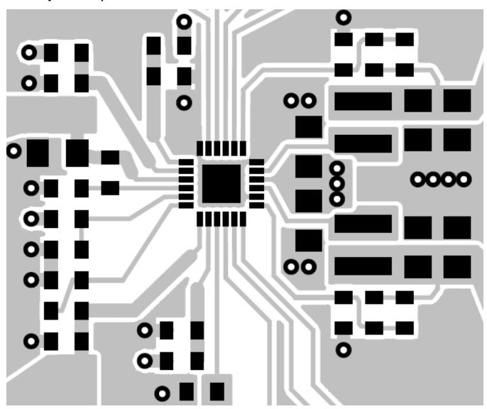
Figure 28. Layout Example Schematic for TPS65053
