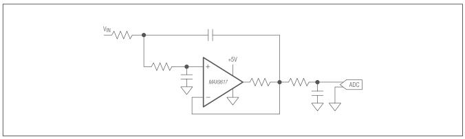
Figure 1. Typical Application Circuit: Sallen-Key Active Lowpass Filter
