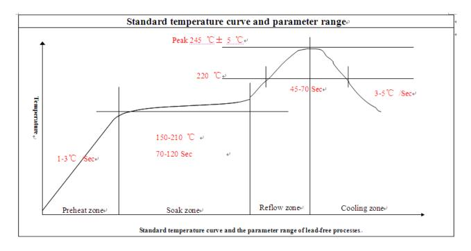
Figure 47: Typical Solder Reflow Profile
