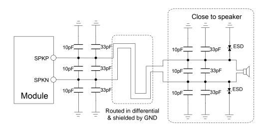
Figure 30: Speaker reference circuit
