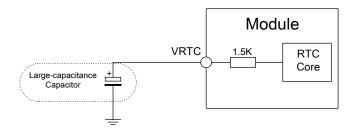
Figure 17: RTC supply from capacitor
