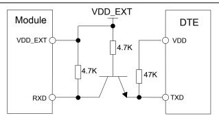
Figure 24: RX level converting by transistor
