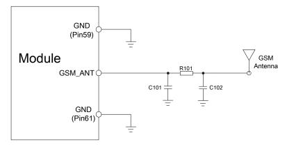
Figure 43: GSM antenna matching circuit without RF connector
