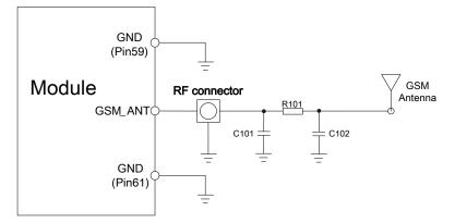
Figure 42: GSM antenna matching circuit
