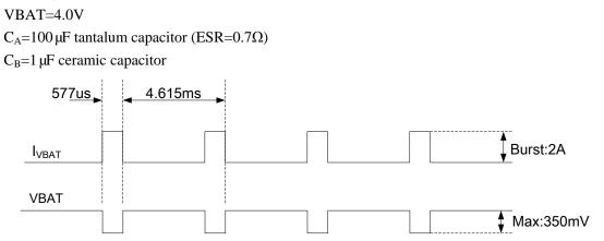
Figure 8: VBAT voltage drop during max power transmitting
