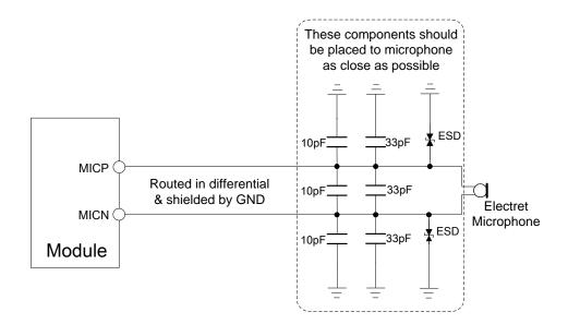
Figure 31 : Microphone reference circuit
