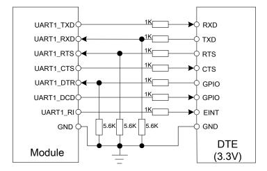
Figure 21: Level converting by resistor
