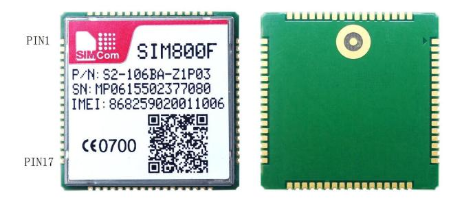
Figure 46: Top and bottom view of SIM800F
