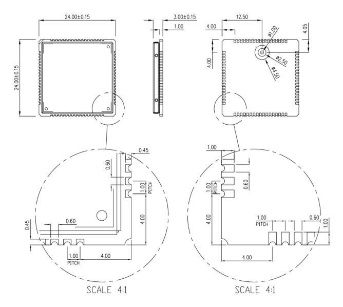
Figure 3: Dimensions of SIM800F (Unit: mm)
