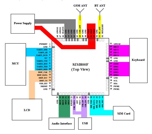
Figure 45: Pin assignment
