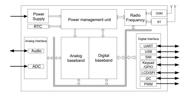
Figure 1: SIM800F functional diagram
