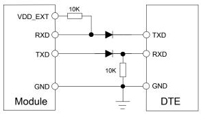
Figure 22: Level converting by diodes
