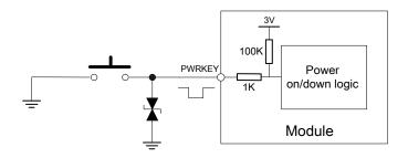
Figure 11: Powered on/down module using button
