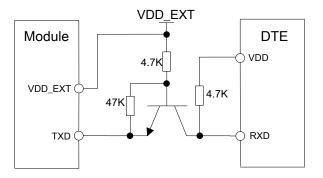
Figure 23: TX level converting by transistor
