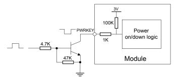
Figure 10: Powered on/down module using transistor
