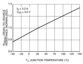
Figure 5. On–Resistance Variation with Temperature
