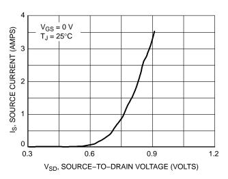
Figure 10. Diode Forward Voltage versus
