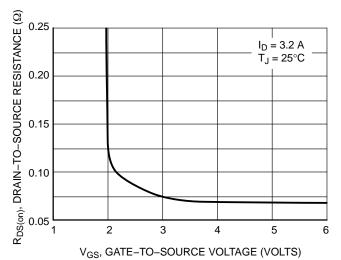
Figure 3. On–Resistance versus Gate–to–Source Voltage
