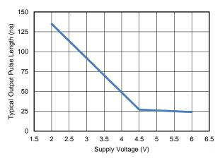
Figure 5. Typical Output Pulse Length Over V<sub>CC</sub> Range
