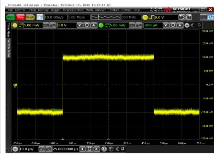
Voltage: 5mV/div, Time: 10μs/div RL=2K, CL=100pF, G=1 Figure 15. 20mV Signal Step Response
