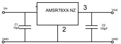
**C1**: A low ESR capacitor is required to keep the noise of the converter to a minimum. Ceramic capacitors are recommended, but tantalum or electrolytic may be used. Typical value is  $10\mu$ F / 50V. **C2**: Installation of C2 is recommended but optional. Typical recommended value is  $100\mu$ F / 25V electrolytic. **NOTE: This part is not designed for parallel operation**
