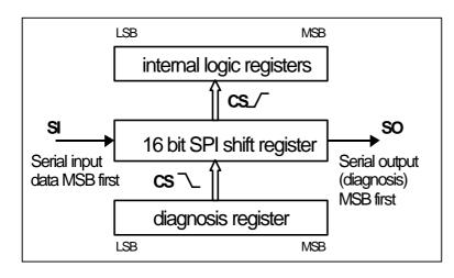
**CS = H:** Any signals at the SCLK and SI pins are ignored and SO is forced into a high impedance state.
