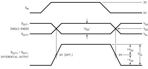
Figure 5. Driver Output Levels
