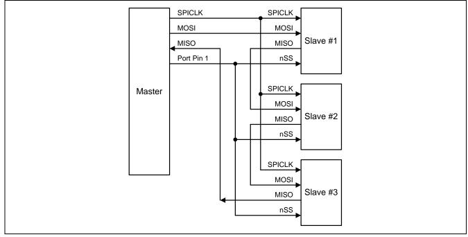
Figure 18–9. SPI slave in Daisy-Chain configuration
