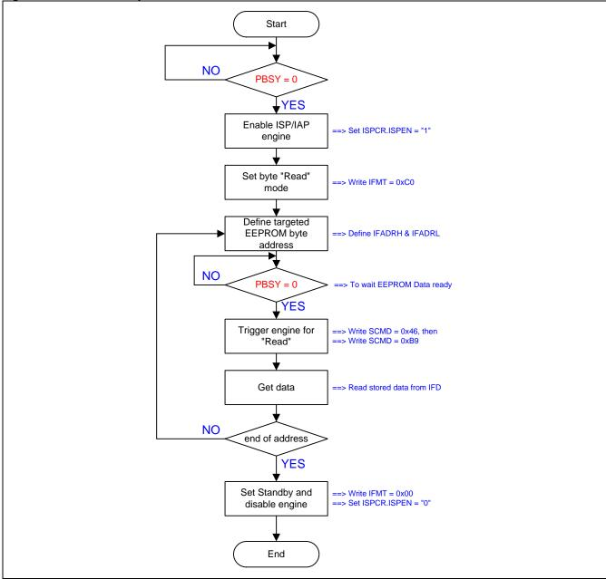
Figure 27–5 shows the demo code of the EEPROM byte read operation.
