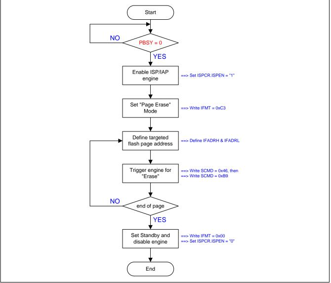
Figure 27–7 shows the demo code of the ISP/IAP page erase operation.
