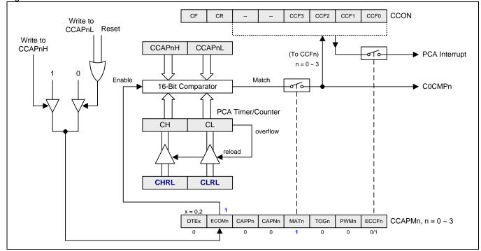
Figure 16–7. PCA Software Timer Mode
