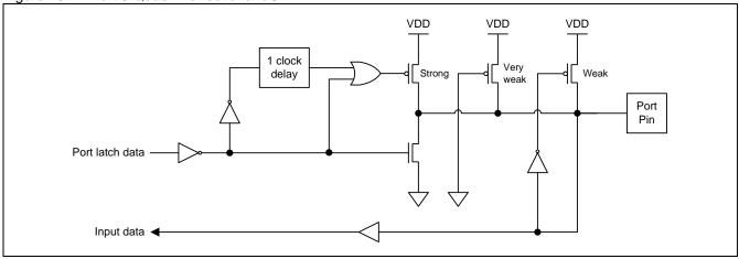
Figure 13-1. Port 3 Quasi-Bidirectional I/O
