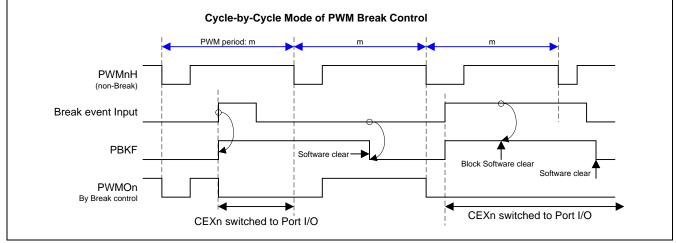
Bit 4~3: <u>PBKE1.1~0</u>, <u>PWM Break Enable 1 selection</u>. This function is only active on CEXn output mode (n=0~3).
