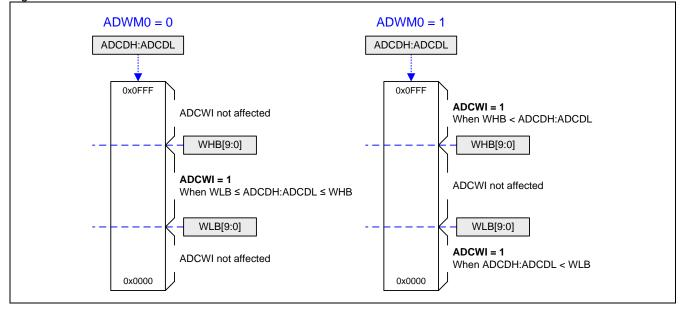
Figure 24–4. ADC Window Detect
