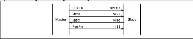
Figure 18–2. SPI single master & single slave configuration
