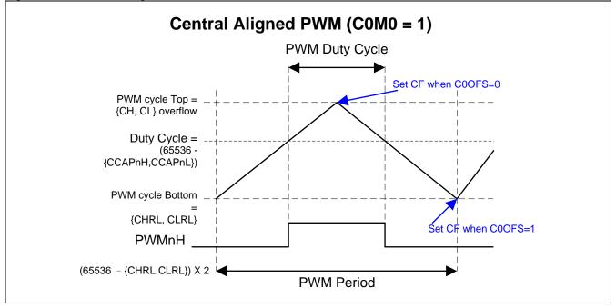
Figure 16-22. Central Aligned PWM with Variable Resolution
