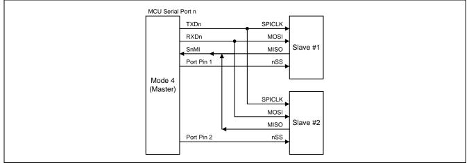
The SPI master satisfies the transfer with the full function SPI module of Megawin MG82/84 series MCU with CPOL, CPHA and DORD selection. For CPOL and CPHA condition, **MG82F6B08 / 6B001/ 6B104** uses an easy way by initialize SPI clock assigned port pin (TXD0) polarity to fit them. Table 17–17 shows the serial port Mode 4 mapping with the four SPI operating mode.
