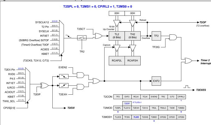
Figure 15–14. Timer 2 Mode 2 Structure (Capture Mode)
