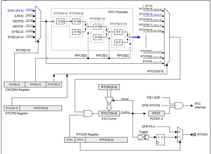
Figure 10-1. Real-Time-Clock Counter
