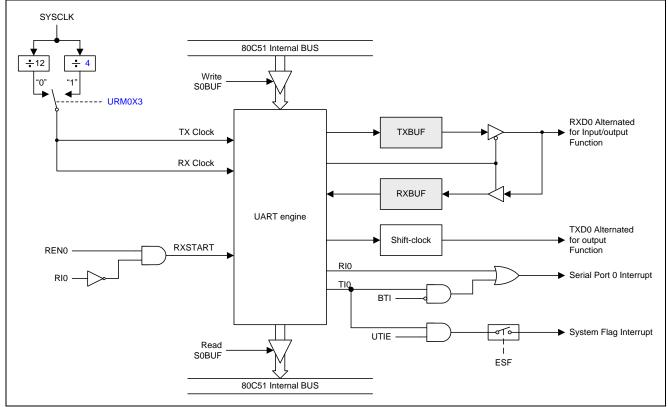
Figure 17-3. Serial Port 0 Mode 0
