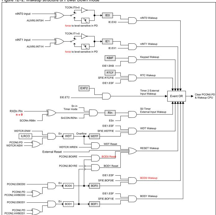
Figure 12–2. Wakeup structure of Power Down mode
