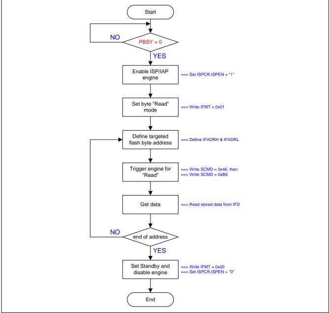
Figure 27–11 shows the demo code of the ISP/IAP byte read operation.
