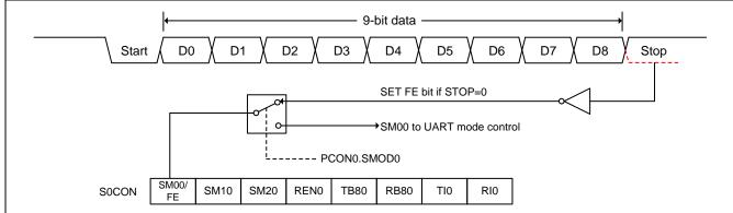
Figure 17–7. UART0 Frame Error Detection
