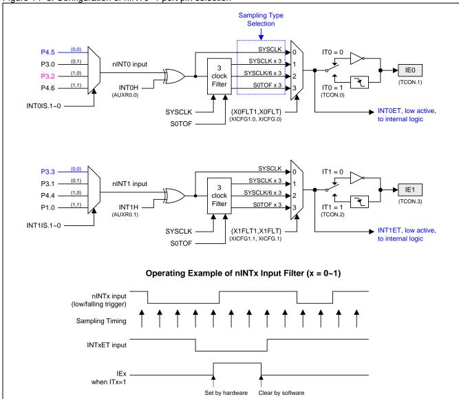
Figure 14-3. Configuration of nINT0~1 port pin selection
