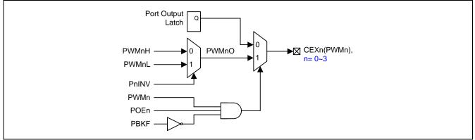
POEM0 in **MG82F6B08 / 6B001/ 6B104** controls the POEn output timing to align with PWM cycle. The configuration and waveform of the aligned function is shown in Figure 16–21.
