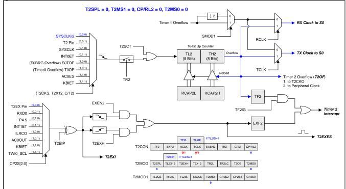
Figure 15–22. Timer 2 in Baud-Rate Generator Mode
