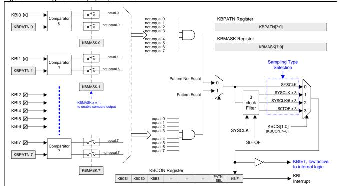
Figure 22–1. Keypad Interrupt (KBI) structure
