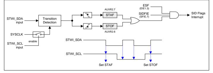
Figure 20–1. Serial Interface Detection structure
