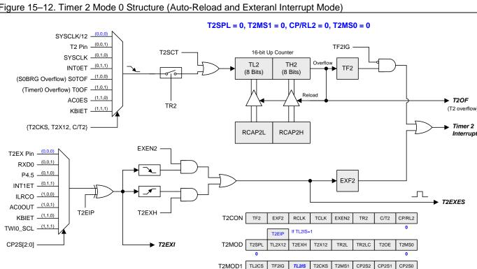
Figure 15–12. Timer 2 Mode 0 Structure (Auto-Reload and Exteranl Interrupt Mode)
