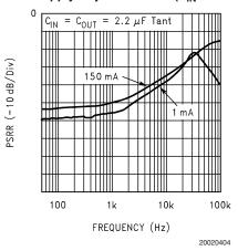
Power Supply Rejection Ratio (V<sub>IN</sub> = 3.5V)
