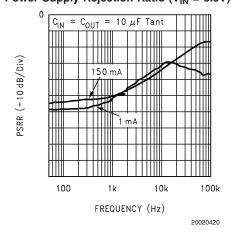
Power Supply Rejection Ratio (LP3984-1.5, V<sub>IN</sub> = 2.5V)
