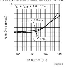
**Typical Performance Characteristics** Unless otherwise specified,  $C_{IN} = C_{OUT} = 1~\mu\text{F}$  Tantalum,  $V_{IN} = 2.5~\text{for}$  1.5, 1.8, and 2.0V options,  $V_{IN} = V_{OUT} + 0.2V$  for output options higher than 2.5V,  $T_A = 25~\text{C}$ , Enable pin is tied to V<sub>IN</sub>. (Continued)
