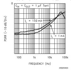
Power Supply Rejection Ratio (V<sub>IN</sub> = 3.5V)
