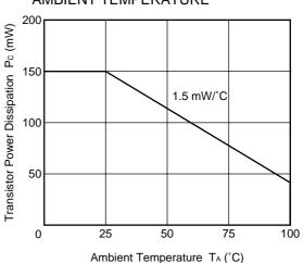
TRANSISTOR POWER DISSIPATION vs. AMBIENT TEMPERATURE
