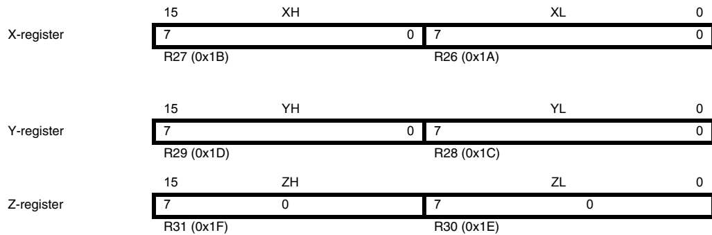
Figure 6-3. The X-, Y-, and Z-registers
