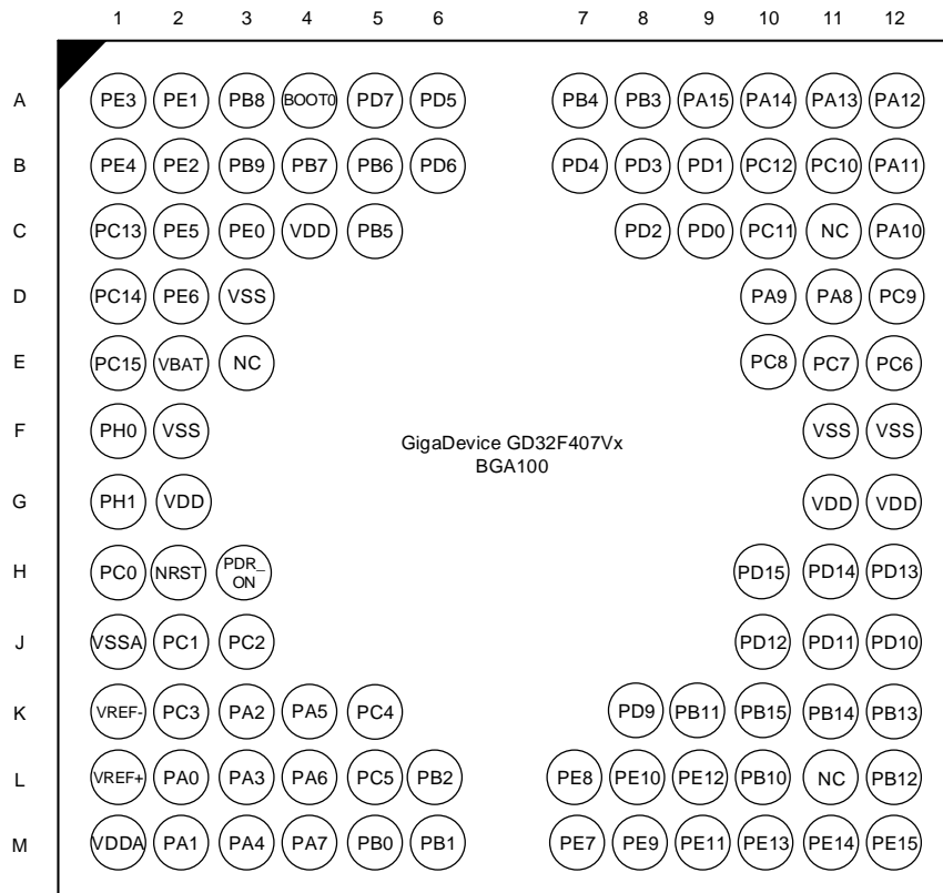
Figure 2-3. GD32F407Vx BGA100 pinouts
