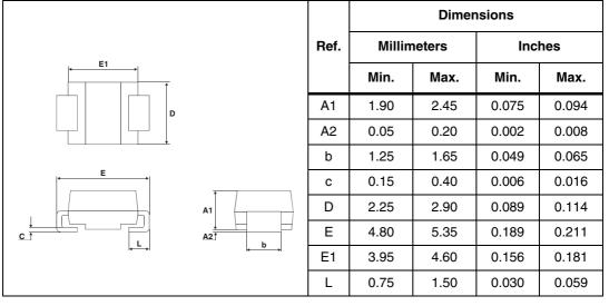
Figure 14. Footprint, dimensions in mm (inches)
