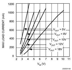
Max. Load Current (typ) vs V<sub>IN</sub> - "X"
