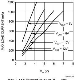
Max. Load Current (typ) vs V<sub>IN</sub> - "Y"
