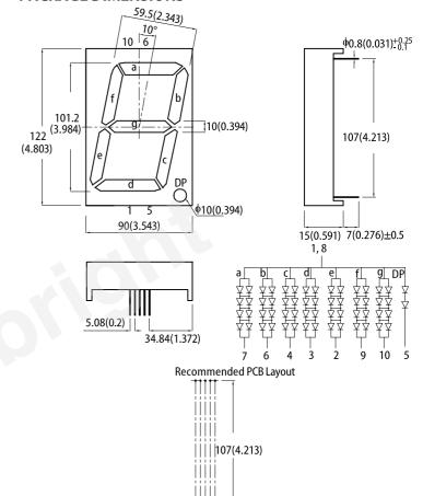
All dimensions are in millimeters (inches), Tolerance is ±0.25(0.01")unless otherwise noted.
