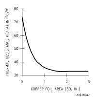
FIGURE 5.  $\theta_{\rm JA}$  vs Copper (1 Ounce) Area for TO-263 package
