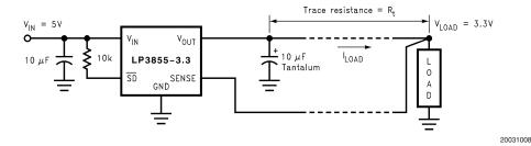
FIGURE 4. Improving remote load regulation using LP3855
