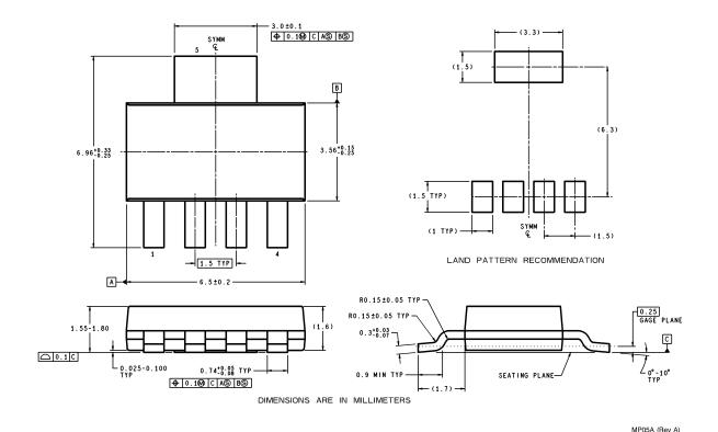
SOT223, 5-Lead, Molded, Surface Mount Package (SOT223-5)
