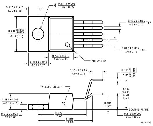
TO220 5-lead, Molded, Stagger Bend Package (TO220-5)
