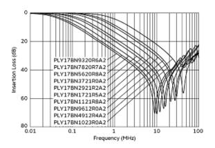
Common Mode Insertion Loss-Frequency Characteristics
