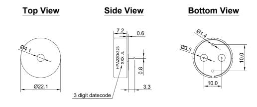
Figure 3. HPA22D/323 Mechanical Layout
