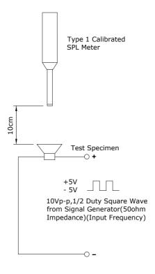
Figure 2. Test Setup
