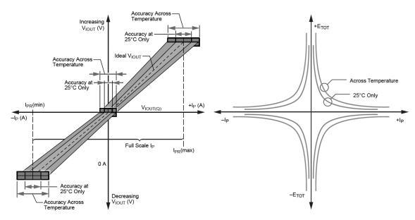
Figure 2: Output Voltage versus Sensed Current
