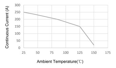
Figure 7: Maximum Continuous Current at a Given TA
