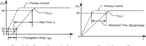
Figure 5: Rise Time and Propagation Delay
