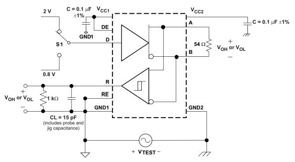
Figure 12. Half-Duplex Common-Mode Transient Immunity Test Circuit
