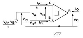
Figure 7. Receiver Voltage and Current Definitions
