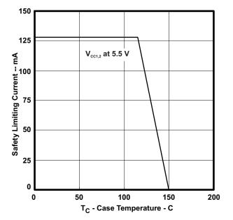
Figure 14. DW-16  $\theta_{\text{JC}}$  Thermal Derating Curve per IEC 60747-5-2
