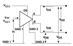
Figure 1. Driver V<sub>OD</sub> Test and Current Definitions
