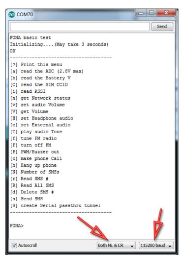
Make sure you also have **Both NL & CR** for the serial command sender option. This means when you send data to the Arduino via the console, it will put a newline/return at the end.
