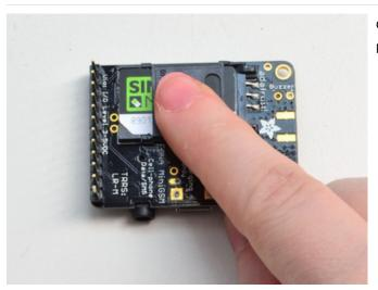
Close the hinge down and slide the cover to lock it in place
