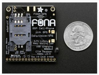
The SIM card holder is on the back. It holds a very-standard "Mini SIM"
