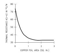
Figure 20.  $\theta_{JA}$  vs Copper (1 Ounce) Area for DDPAK/TO-263 Package
