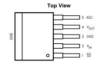
Figure 2. DDPAK/TO-263-5 Package See Package Number KTT0005B
