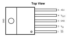
Figure 1. TO-220-5 Package Bent, Staggered Leads See Package Number NDH0005D
