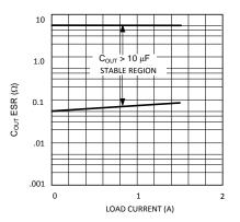
Figure 18. ESR Curve for C<sub>OUT</sub> (with 10µF Tantalum Input Capacitor)
