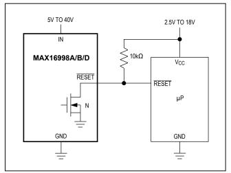
Figure 9. Interfacing to Other Voltage Levels
