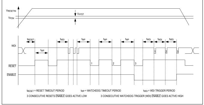
Figure 2. MAX16998A Timing Diagram
