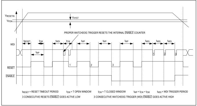
Figure 3. MAX16998B/D Timing Diagram
