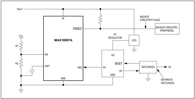
Figure 12. MAX16997A Application Diagram
