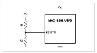
Figure 7. Setting RESETIN Voltage for the MAX16998A/B/D
