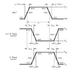
FIGURE 3. AC Waveforms
