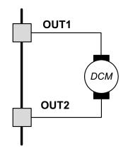
Figure 7. Single DC Motor Connection
