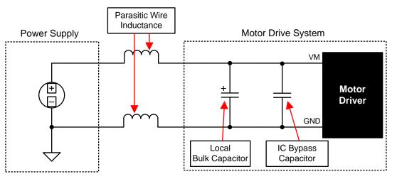
Figure 12. Bulk Capacitance
