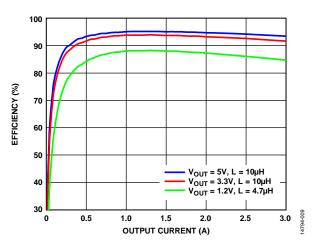
Figure 9. Efficiency at  $V_{IN} = 12 \text{ V}$ ,  $f_{SW} = 300 \text{ kHz}$
