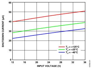
Figure 11. Shutdown Current vs. Input Voltage (V<sub>PVIN</sub>)
