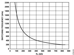
Figure 33. Switching Frequency vs. R<sub>T</sub>
