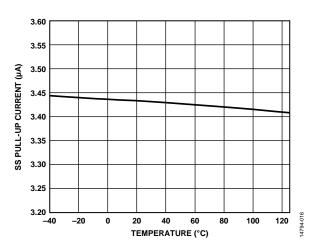
Figure 16. SS Pin Pull-Up Current vs. Temperature
