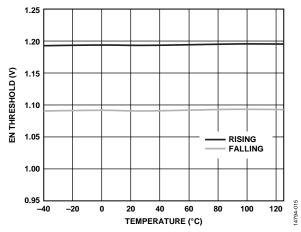
Figure 15. EN Threshold vs. Temperature
