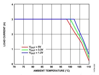
Figure 30. Load Current vs. Ambient Temperature at  $V_N$  = 12 V,  $f_{SW}$  = 600 kHz, Measured on ADP2443-EVALZ
