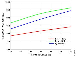
Figure 14. Quiescent Current vs. Input Voltage (V<sub>PVIN</sub>)
