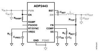
Figure 41. High Current Path in the PCB Circuit
