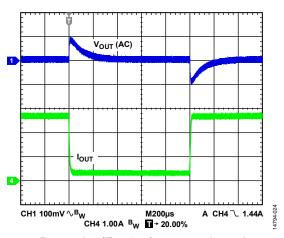
Figure 24. Load Transient Response, 0.3 A to 2.7 A
