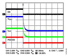
Figure 26. Shutdown with Full Load
