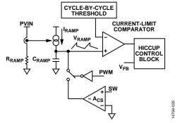
Figure 35. Current-Limit Circuit
