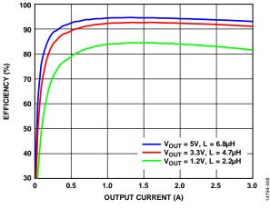
Figure 8. Efficiency at  $V_{IN} = 12 \text{ V}$ ,  $f_{SW} = 600 \text{ kHz}$
