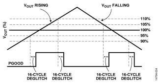
Figure 34. PGOOD Rising and Falling Thresholds
