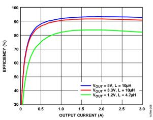
Figure 6. Efficiency at  $V_{IN} = 24 \text{ V}$ ,  $f_{SW} = 300 \text{ kHz}$
