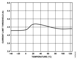
Figure 21. Current-Limit Threshold vs. Temperature
