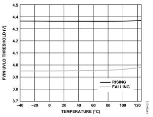
Figure 12. PVIN UVLO Threshold vs. Temperature
