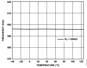
Figure 20. Frequency vs. Temperature
