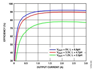
Figure 5. Efficiency at  $V_{IN} = 24 \text{ V}$ ,  $f_{SW} = 600 \text{ kHz}$
