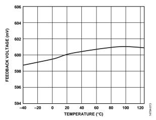
Figure 13. Feedback Voltage vs. Temperature
