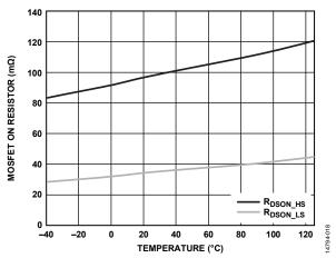
Figure 18. MOSFET On Resistor vs. Temperature
