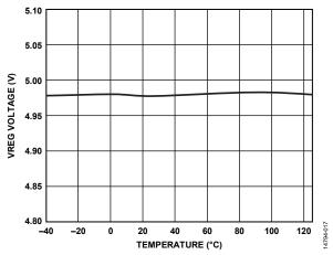
Figure 17. VREG Voltage vs. Temperature
