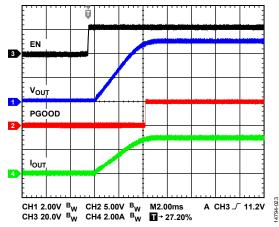
Figure 23. Soft Start with Full Load
