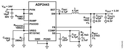
Figure 43. Typical Application Circuit,  $V_{IN} = 24 \text{ V}$ ,  $V_{OUT} = 3.3 \text{ V}$ ,  $I_{OUT} = 3A$ ,  $f_{SW} = 600 \text{ kHz}$
