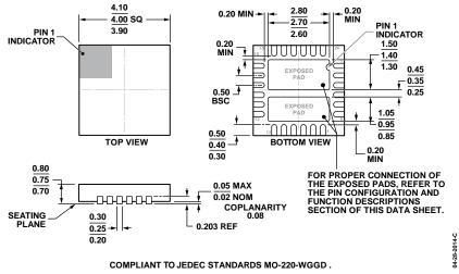
Figure 46. 24-Lead Lead Frame Chip Scale Package [LFCSP] 4 mm × 4 mm Body and 0.75 mm Package Height (CP-24-12) Dimensions shown in millimeters
