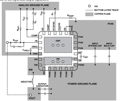
Figure 42. Recommended PCB Layout Rev. 0 | Page 22 of 24
