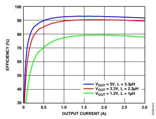
Figure 10. Efficiency at  $V_{IN} = 12 \text{ V}$ ,  $f_{SW} = 1.2 \text{ MHz}$
