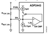
Figure 37. Programming the Input Voltage UVLO
