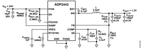
Figure 44. Programming Input Voltage UVLO Rising Threshold at 20 V, Falling Threshold at 18 V,  $V_{IN} = 24$  V,  $V_{OUT} = 1.2$  V,  $I_{OUT} = 3$  A,  $I_{SW} = 500$  kHz
