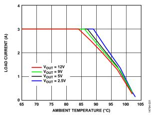
Figure 31. Load Current vs. Ambient Temperature at  $V_N$  = 36 V,  $f_{SW}$  = 600 kHz, Measured on ADP2443-EVALZ
