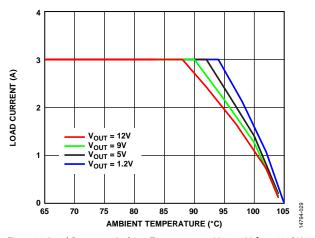
Figure 29. Load Current vs. Ambient Temperature at  $V_{IN}$  = 24 V,  $f_{SW}$  = 600 kHz, Measured on ADP2443-EVALZ
