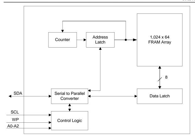
Figure 1. FM24C64 Block Diagram
