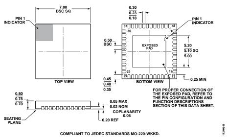
Figure 15. 48-Lead Lead Frame Chip Scale Package [LFCSP] 7 mm × 7 mm Body and 0.75 mm Package Height (CP-48-4) Dimensions shown in millimeters
