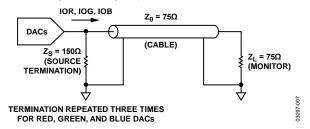
Figure 9. Analog Output Termination for RS-170
