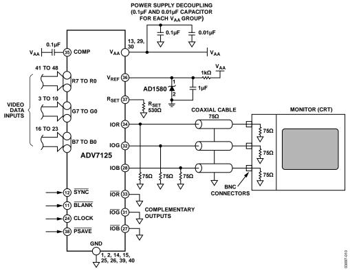
Figure 12. Typical Connection Diagram
