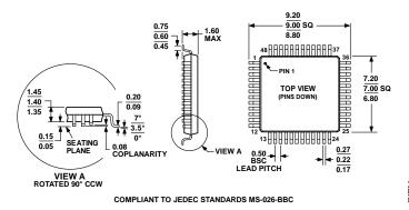
Figure 13. 48-Lead Low Profile Quad Flat Package [LQFP] (ST-48) Dimensions shown in millimeters
