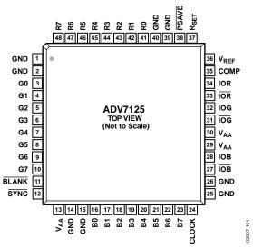
Figure 5. LQFP Pin Configuration
