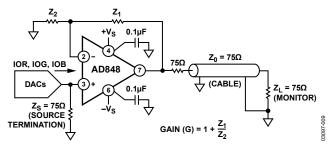
Figure 11. AD848 as an Output Buffer
