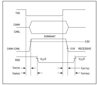
Figure 2. Timing Diagram for Dynamic Characteristics
