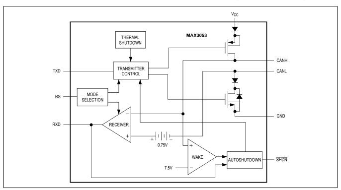
Figure 4. Block Diagram
