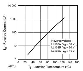
Fig. 3 - Reverse Current vs. Junction Temperature
