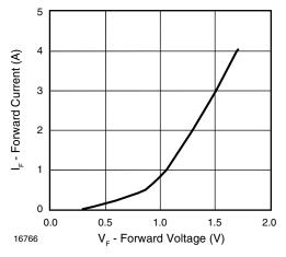
Fig. 2 - Forward Current vs. Forward Voltage
