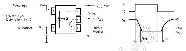
Test Circuit 2: Common Mode Transient Immunity Test Circuit
