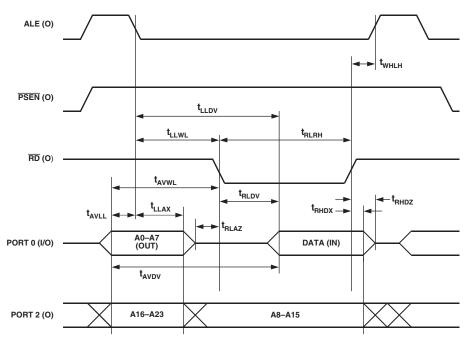
Figure 72. External Data Memory Read Cycle
