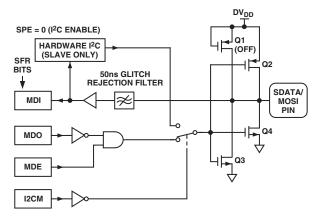
Figure 45. SDATA/MOSI Pin I/O Functional Equivalent in I<sup>2</sup>C Mode
