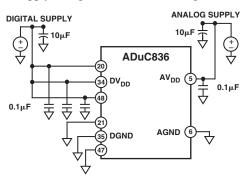
Figure 61. External Dual-Supply Connections
