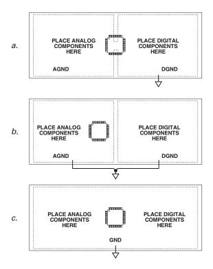
Figure 64. System Grounding Schemes
