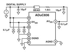
Figure 62. External Single-Supply Connections
