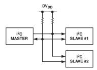
Figure 35. Typical I<sup>2</sup>C System
