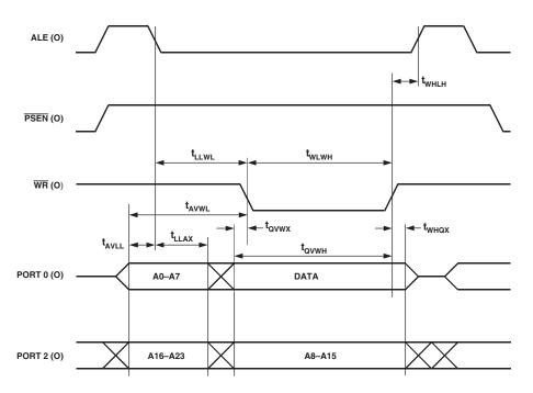
Figure 73. External Data Memory Write Cycle
