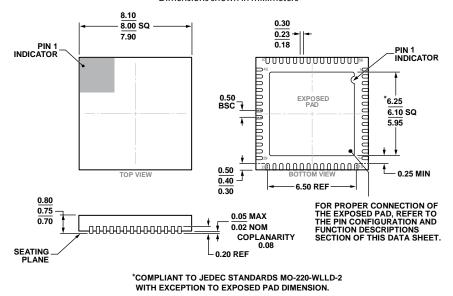
Figure 81. 56-Lead Lead Frame Chip Scale Package [LFCSP] 8 mm × 8 mm Body and 0.75 mm Package Height (CP-56-11) Dimensions shown in millimeters
