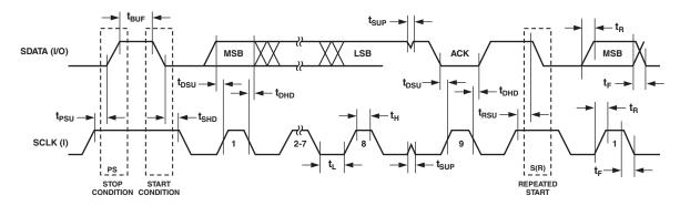
Figure 79. I<sup>2</sup>C Compatible Interface Timing
