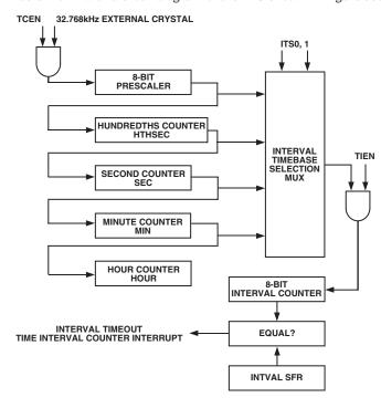
Figure 33. TIC, Simplified Block Diagram
