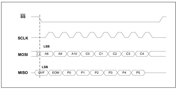
**FIGURE 6: 8-BIT COMMAND FORMAT**
