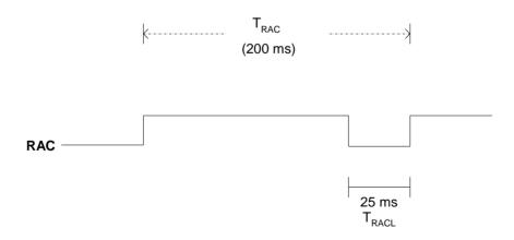
FIGURE 2: RAC TIMING WAVEFORM DURING NORMAL OPERATION
