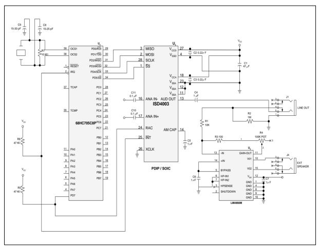
FIGURE 9: APPLICATION EXAMPLE USING SPI
