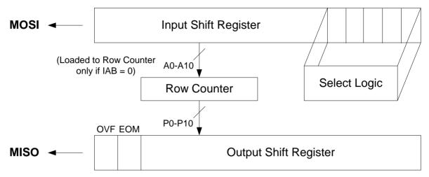
FIGURE 3: SPI INTERFACE SIMPLIFIED BLOCK DIAGRAM
