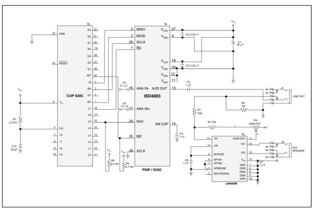
FIGURE 10: APPLICATION EXAMPLE USING MICROWIRE
