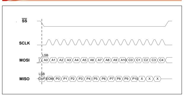
**FIGURE 7: 16-BIT COMMAND FORMAT**
