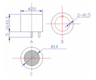
A—Left view B—upward view C—vertical view W electrode — working electrode for oxidation reaction C electrode —counter electrode for deoxidization reaction
