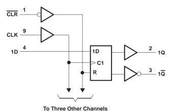
Pin numbers shown are for the D, DB, DGV, J, NS, PW, and W packages.
