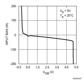
FIGURE 7. Input Bias Current vs.  $V_{\rm CM}$
