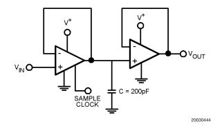
FIGURE 2. Sample and Hold Circuit
