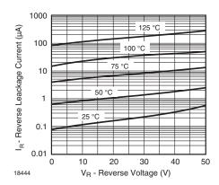
Fig. 3 - Typical Reverse Characteristics
