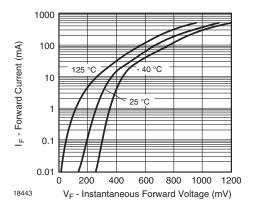
Fig. 2 - Typical Forward Characteristics
