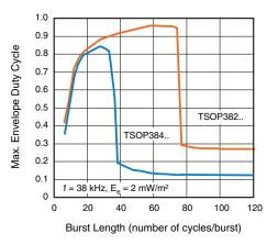
Fig. 8 - Max. Envelope Duty Cycle vs. Burst Length
