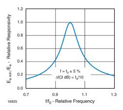
Fig. 5 - Frequency Dependence of Responsivity
