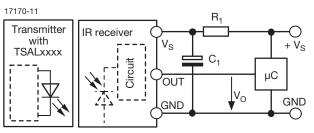
$\rm R_1$  and  $\rm C_1$  recommended to reduce supply ripple for  $\rm V_S$  < 2.8 V
