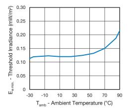
Fig. 9 - Sensitivity vs. Ambient Temperature
