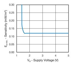
Fig. 13 - Sensitivity vs. Supply Voltage
