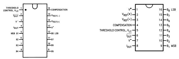
Figure 2. PDIP, CDIP Packages - Top View (See Package Number NFG0016E or NFE0016A)
