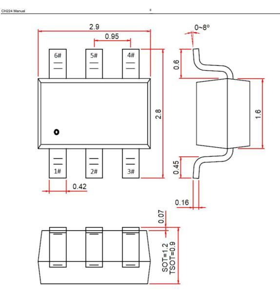
Note: The unit marked in the package information diagram is mm (millimeter).
