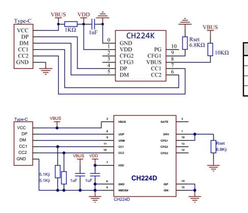
6.2. CH224K uses Type-C female port, the level configuration is 5/9/12/15/20V (the level configuration in the figure is 12v)
