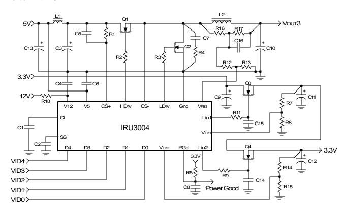
Figure 4 - Typical application of IRU3004 in a Pentium with AGP where the power dissipation of the 3.3V linear regulator is equally distributed between Q3 and Q4 pass transistors. This equal distribution is possible by accurately regulating the first regulator using the IRU3004 linear controller and its internal 1% reference voltage while the second controller regulates the output of the first regulator from 4.17V to 3.3V, thereby distributing the power dissipation equally.
