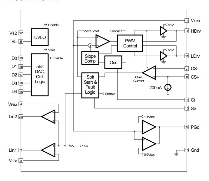
Figure 2 - Simplified block diagram of the IRU3004.
