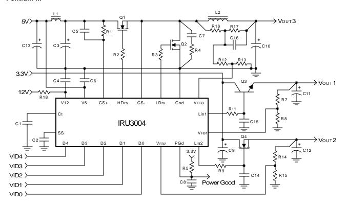
Figure 3 - Typical application of IRU3004 in an on-board DC-DC converter providing the Core, GTL+, and Clock supplies for the Pentium II microprocessor.
