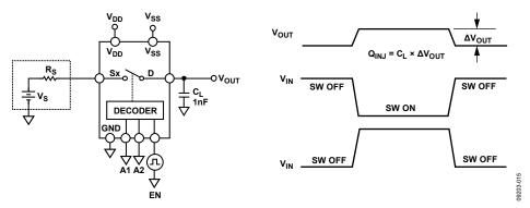
Figure 33. Charge Injection
