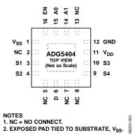
Figure 3. LFCSP Pin Configuration
