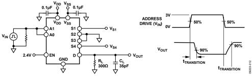
Figure 30. Address to Output Switching Times
