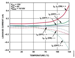
Figure 14. Leakage Currents vs. Temperature, 12 V Single Supply
