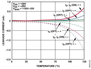
Figure 13. Leakage Currents vs. Temperature, ±20 V Dual Supply
