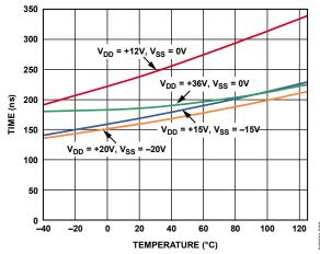
Figure 20. Transition Time vs. Temperature
