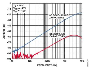
Figure 21. ACPSRR vs. Frequency, ±15 V Dual Supply
