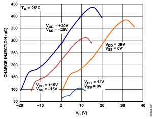
Figure 19. Charge Injection vs. Source Voltage
