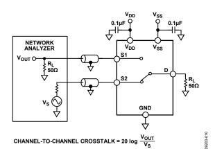
Figure 28. Channel-to-Channel Crosstalk
