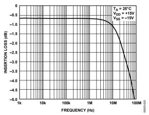
Figure 18. On Response vs. Frequency, ±15 V Dual Supply
