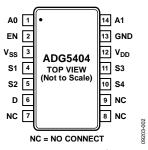
Figure 2. TSSOP Pin Configuration
