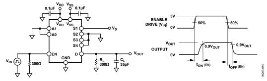
Figure 32. Enable-to-Output Switching Delay
