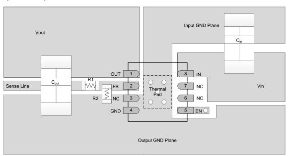
Figure 15. Recommended Layout Example
