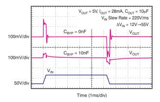
Figure 14. Line Transient Response vs CBYP
