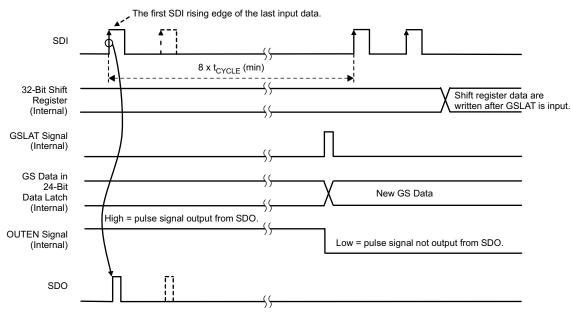
Figure 16. GS Data Latch Sequence (GSLAT)
