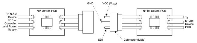
Figure 11. Connector Pin Design Application
