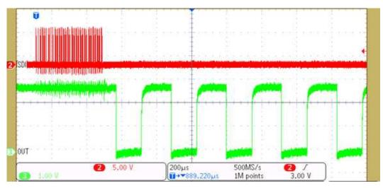
Figure 22. Output Waveform Without GS Data Latch Input
