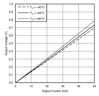
Figure 4. Output Current vs Output Voltage (Outn)
