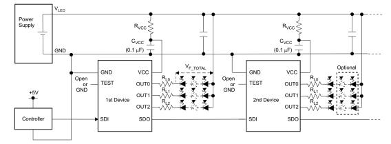
Figure 10. Internal Shunt Regulator Mode Application Circuit
