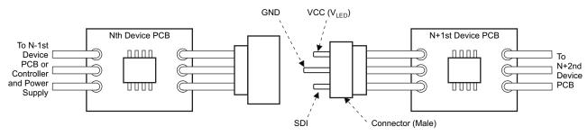
Figure 25. Connector Pin Design Application
