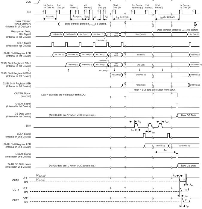
(1) OUT*n* ON-time changes, depending on the data in the 24-bit GS data latch.
