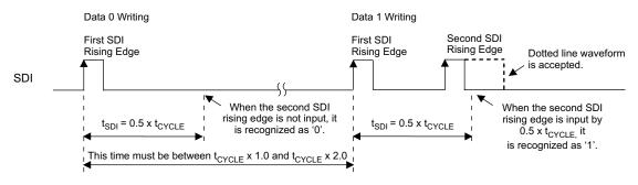
Figure 14. Data 0 and 1 Write Operation
