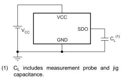
Figure 9. Rise Time and Fall Time Test Circuit for SDO
